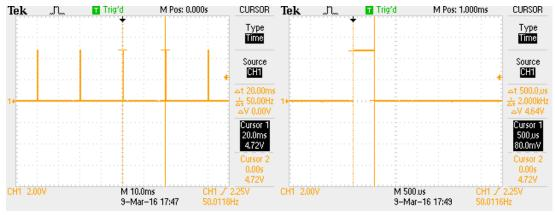
When control port is 90°, the oscillo-gram is the pic below (the pic on the right is enlarged drawing of a single wave).
