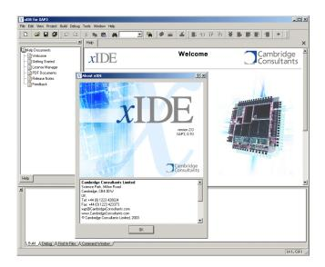
xIDE is a flexible, extensible software development and debug environment for ASICs or embedded systems. It is used to build application development toolsets for ASICs that semiconductor companies can use and also distribute to their customers.
