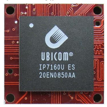
The unique architecture and on-chip hardware engines enable the processor to service various network processing tasks simultaneously without sacrificing line rate performance or Quality of Service (QoS). With core power consumption in the range of 0.5W for routing applications, the IP71xx network processor family offers high performance and low power CPU with extremely low price points.
